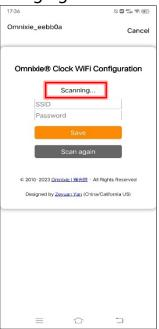
If Wi-Fi configuration interface does not pop up automatically, please open browser and type **192.168.4.1** to open Wi-Fi configuration interface.
