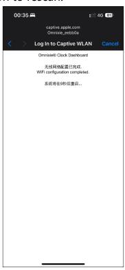
After the Wi-Fi configuration is completed, the clock will reboot and connect to the Wi-Fi automatically. If the connection is successful, the Wi-Fi status indicator will light **yellow** or **green**. If Wi-Fi status indicator still red after rebooting, it indicates that the Wi-Fi password just entered is incorrect, please select again to make settings.
